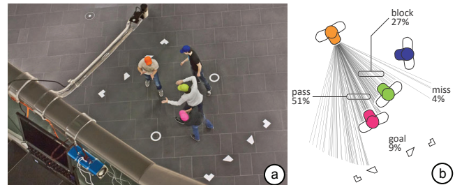
Figure 3: (a) In this game of Quantum team handball, the orange player is trying to pass the ball to his pink teammate. (b) The underlying game engine represents the ball as a set of particles each representing one plausible ball trajectory.
