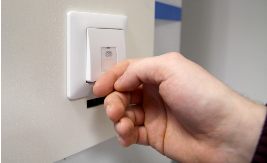
Fig. 6.3 This button enables a low-effort way of user recognition by observing button pressing behavior. For small groups of users, establishing who, e.g., entered a room can then be as easy as pressing a button. In addition to conflating the action with the recognition, this allows for recognition in the periphery as the button can, e.g., be pressed while entering the room.
