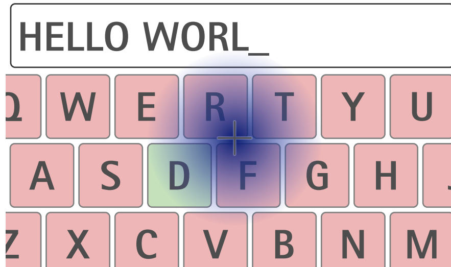
Fig. 6.6 In a touchscreen keyboard a language model provides a probability for the next letter (shown here as key color) and a touch model gives a measure of certainty for a user's touch (here shown as a gradient around the touch position indicated by a cross). The combination of both models determines the most likely next letter. We vary how much influence the language model has by changing the size of the touch area. When users press harder it shrinks and keys closer to the touch are much more likely to be chosen. As users relax and only press lightly, the area increases and many more keys are potentially chosen—increasing the influence of the language model.
