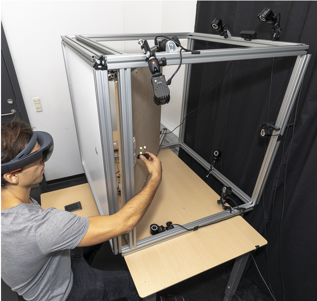
Figure 4: During the study, participants were seated in front of a 1 m 3 frame. They reached in from the right side and interacted with objects placed on a wall, that was tilted at a 30° angle. Movement inside the frame was tracked with an Optitrack setup and participants received visual feedback in a HoloLens headset.
