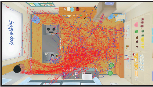
Figure 6. We evaluated the “Who Put That There” system in a 22-minute spatial recording of a kitchen. The blue trajectories show all the objects’ movement through the recording and the red trajectories the two avatars’ movement.
