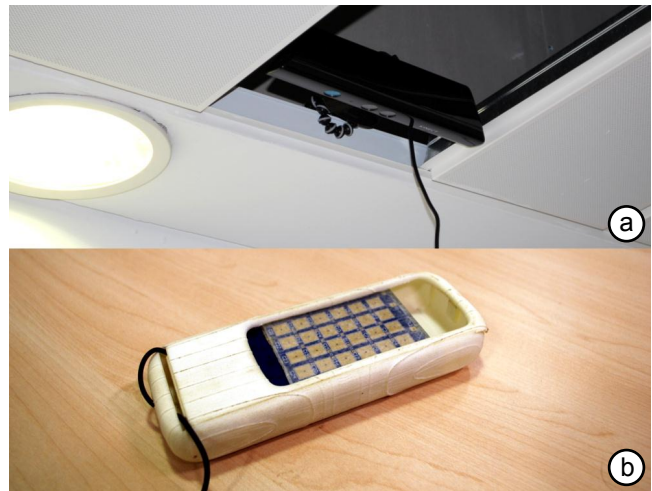
Figure 5. (a) Ceiling mounted Kinect and (b) SHAKE SK7-ExtCS1 capacitive sensing extension board used for the study prototype. This setup allowed for the necessary on and above the device sensing.
