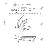
**Figure 1:** In this example, a user can pick the color of a moodlight at varying levels of control. It enables (a) fine control via touch on the device, (b) in-air control of brightness and hue by moving and rotating the hand, and (c) abstract control of mood by waving over the device.
