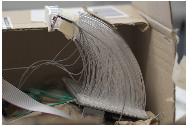
Figure 4: Glass fibers reroute the light from a large LED dot-matrix below the device to our edge display. This allows prototyping with denser LED grids than readily available ones.
