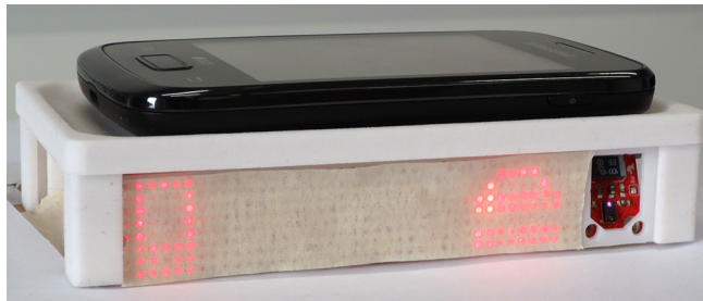
Figure 2: Our prototype consists of a dot-matrix LED display and a proximity sensor mounted underneath a phone.
