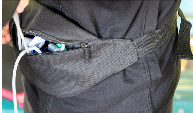
Figure 7: While running, participants carried the compression feedback device and a battery pack around in a pouch. It connects to a strap worn on the leg.
