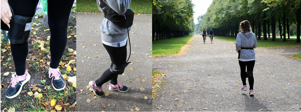
Figure 6: We created a jogging game where runners are pushed to reach checkpoints in a given time via compression feedback. Runners wear a compression feedback strap around one knee. The strap is controlled from a controller board in a waist bag.
